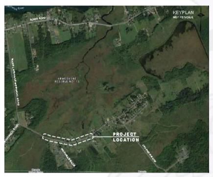
The construction zone will start from the Bittern Creek Bridge to a length of approximately 600m east on Wade Lafrance Memorial Road. The work consists of removing the existing asphalt material and raising the road surface approximately 150mm with granular A.
