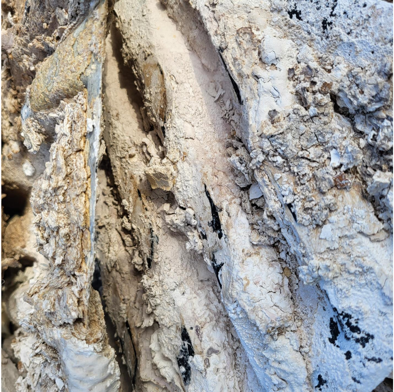
Another media sheet from bank one with extremely heavy alum overloading
